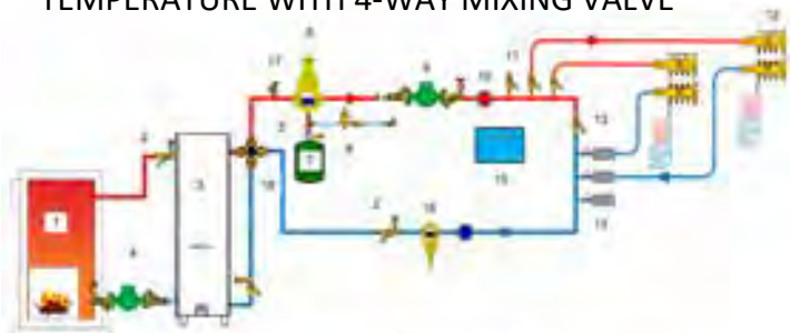
PRESSURIZED WOOD OR COAL BOILER, SINGLE TEMPERATURE WITH 4-WAY MIXING VALVE
