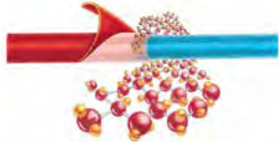
BPEX'S CROSS-LINKING CREATES BONDS BETWEEN INDIVIDUAL MOLECULAR STRANDS, GREATLY ENHANCING THE TUBE'S TEMPERATURE AND CHEMICAL RESISTANCE.
